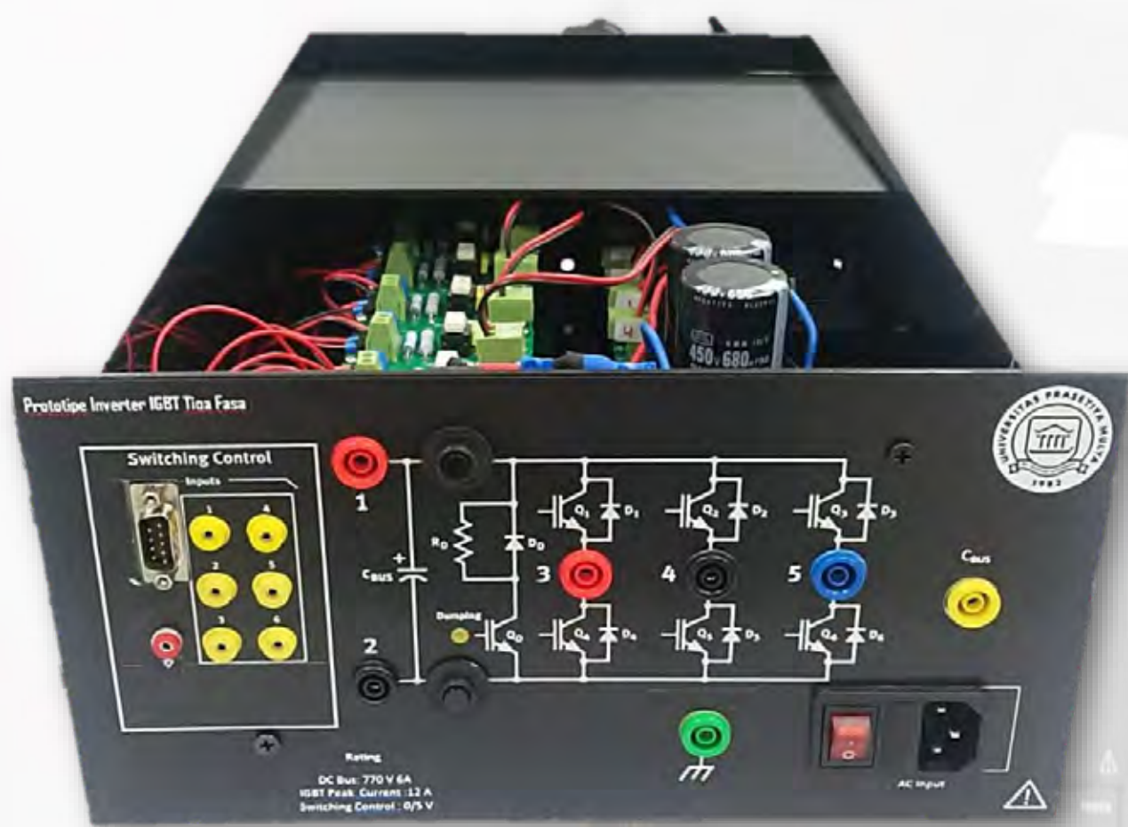
Prototipe Inverter Tiga Fasa berbasis IGBT 25N120
