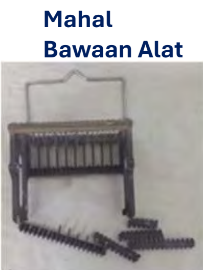
1. Rak Slide Automatic Staining Machine Patah/ Rusak
