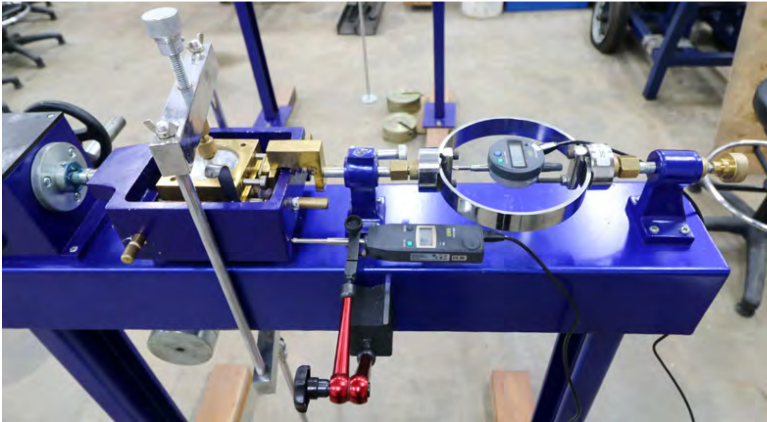
Gambar 2. Alat Direct Shear Test Hasil Inovasi
